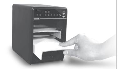
Slide the 4 HDDs into the enclosure and make sure they are securely installed in order from up to down.
